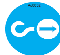
Picture 58: indication of frame coupling.
