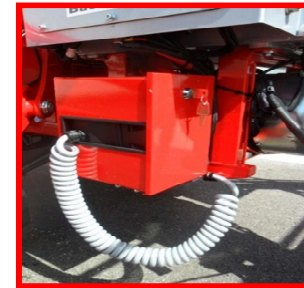
Picture 7: location for remote wired control.
