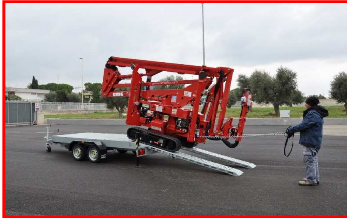
Picture 13: loading/uploading through ramp by wired remote control.
