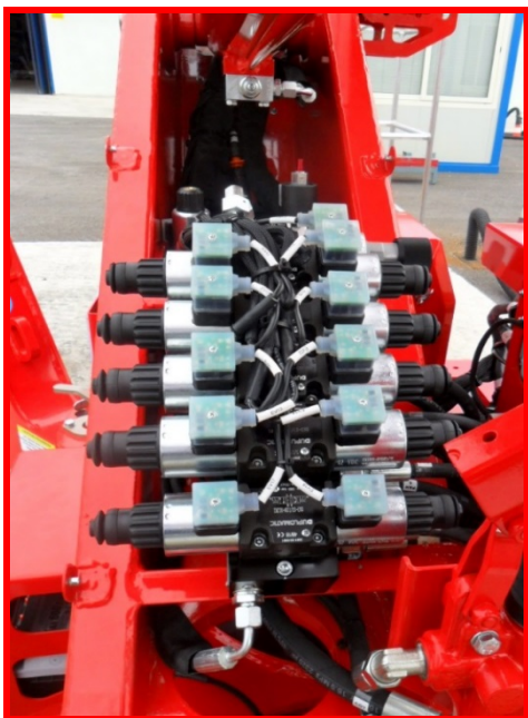
Picture 15: emergency workbench with the main hydraulic distributor.
