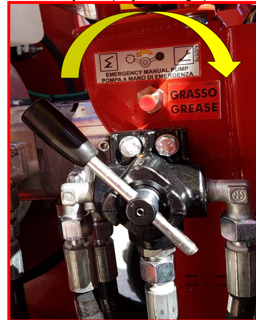
Picture 25: manual pump tap to be turned to the right.
