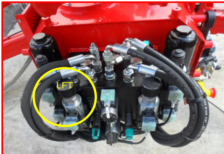
Picture 22: left tap of filters bench.
