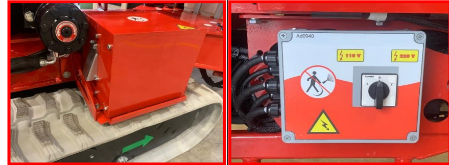
Picture 7a: alternator and selector (*optional).
