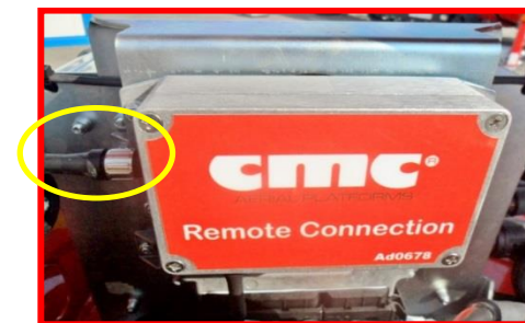
Picture 88: remote connection system.
