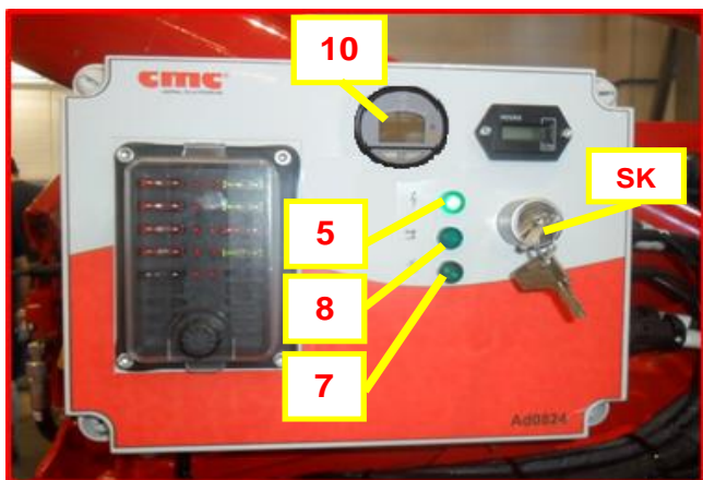
Picture 4b: machine switching on/off station in case of full lithium version.
