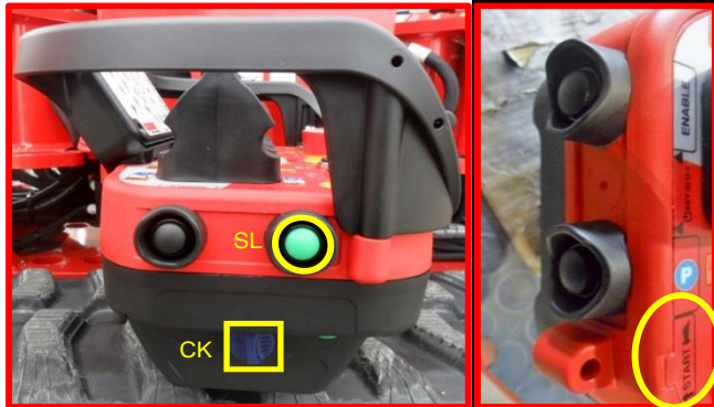
Picture 8a: start/link button on radio control.
