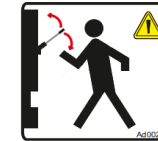
Picture 70: indication of emergency manual pump.
