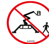
Picture 51: prohibition to stand in work area.
