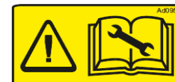
Picture 83: warning to obligate to the consultation of use and maintenance manual.
