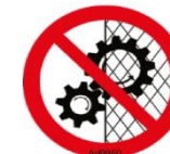
Picture 52: prohibition to remove safety devices.
