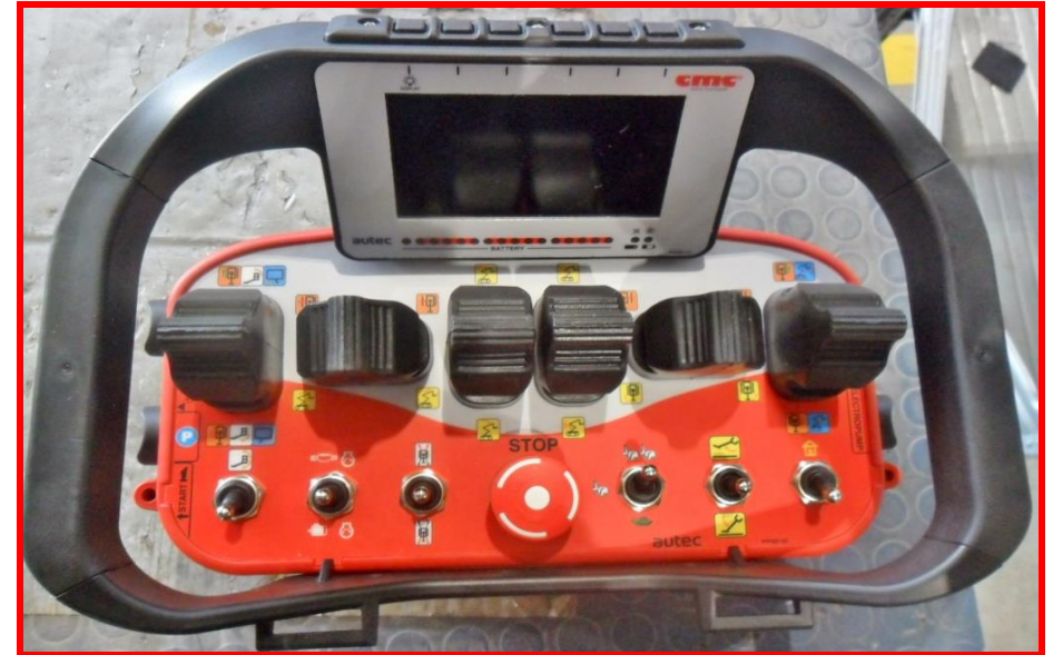
Picture 13: platform radio control station.
