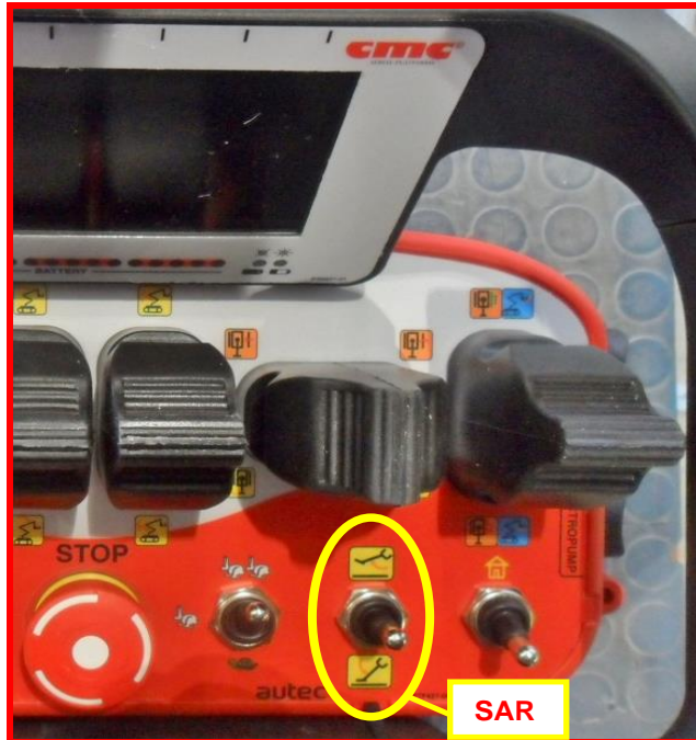
Picture 48: stabilization/destabilization lever on radio control.
