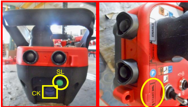
Picture 14: start/link button on radio control.
