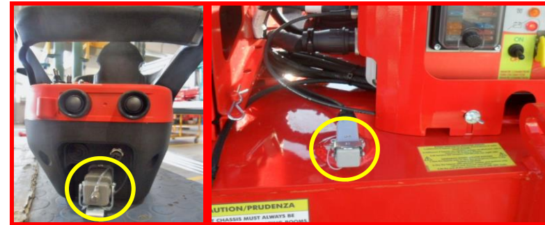
Picture 17: radio control connection.
