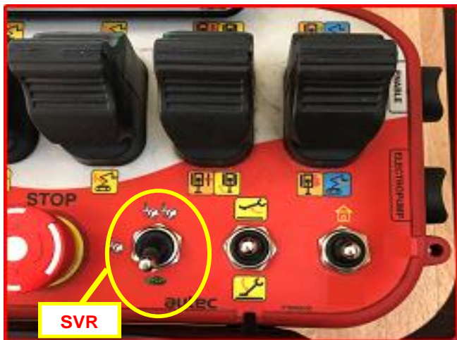
Picture 43: speed selector on travel radio control.
