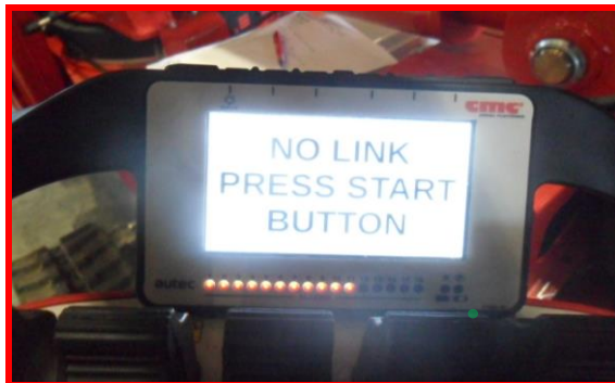
Picture 15: no link message on radio control display.
