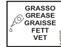
Picture 90: indication for grease application.
