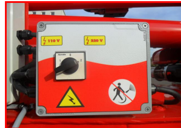
Picture 8b: transformer box with voltage selector.
