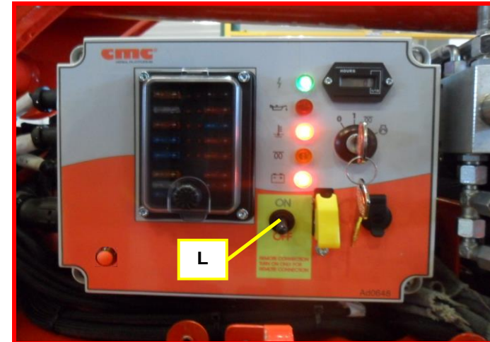
Picture 121: chassis box.
