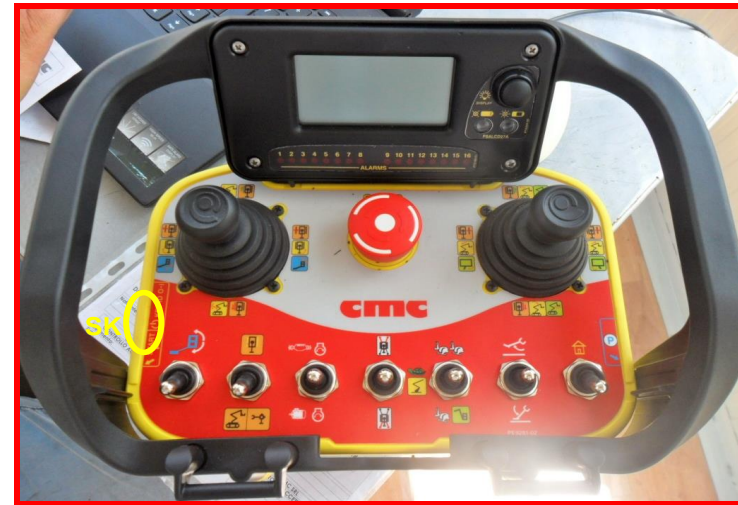
Picture 13: platform wired remote/radio control station.
