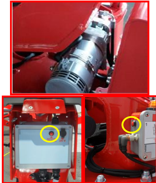
Picture 41: electropump (*optional) activation buttons.
