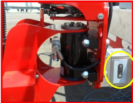
Picture 29: load cell.
