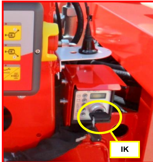
Picture 4: engine switch on/off station if Kubota.
