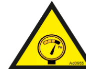
Picture 87: high pressure hazard.
