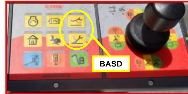
Picture 27: stabilization/destabilization buttons on basket station control.
