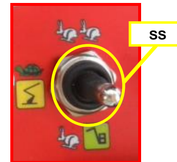
Picture 22: speed selector on wired remote control.
