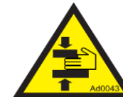
Picture 86: crushing and cutting hazard.
