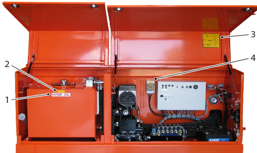
Hydraulic oil and valve/electrical compartment
