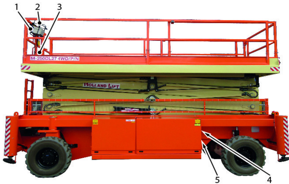
Overview of the controls
