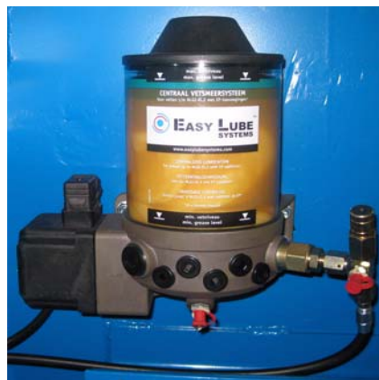
Easy Lube Systems™ grease reservoir
