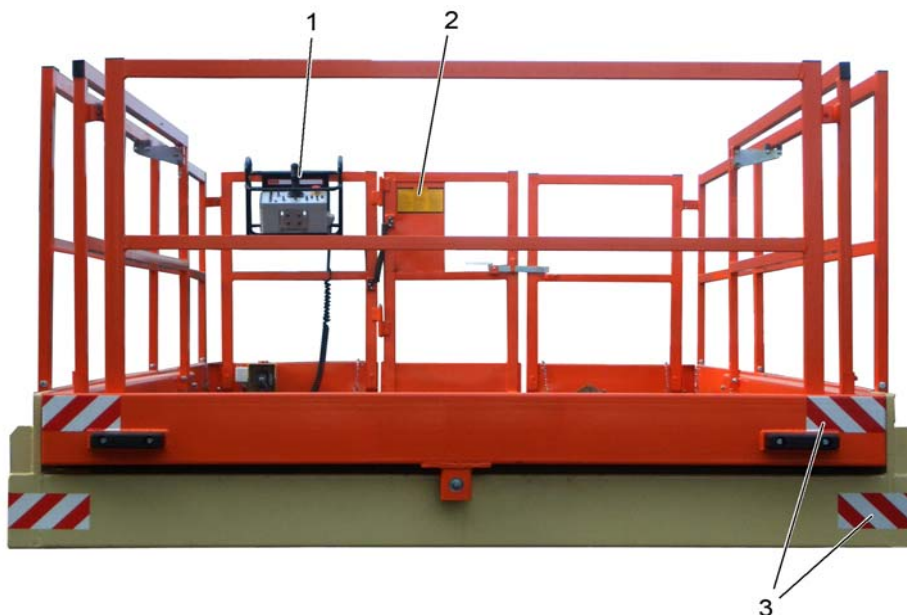
Decalls on the inside of the platform
