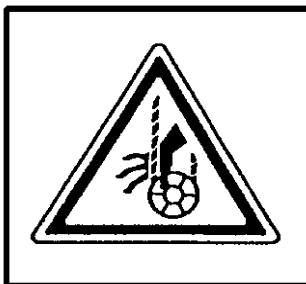
(25) Caution against being entangled by the hook block (553-4267400)
