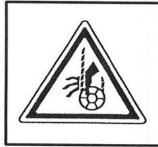
(15) Hook Block Winding Caution (553-4267400) (2 places)
