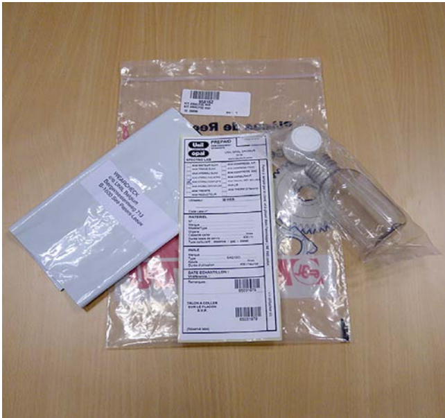
Figure 173: Hydraulic oil contamination check
