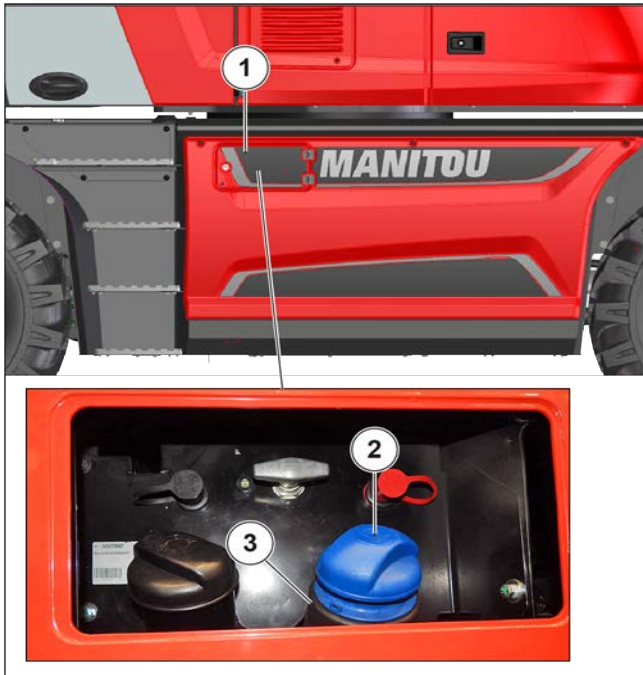
Figure 149: Checking DEF liquid level
