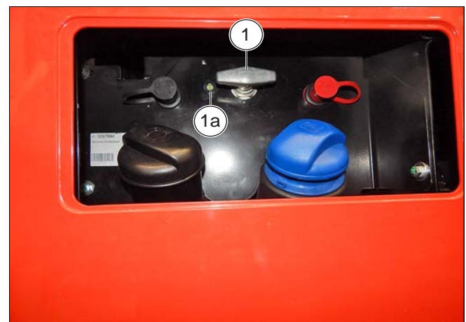
Figure 66: Battery disconnect switch
