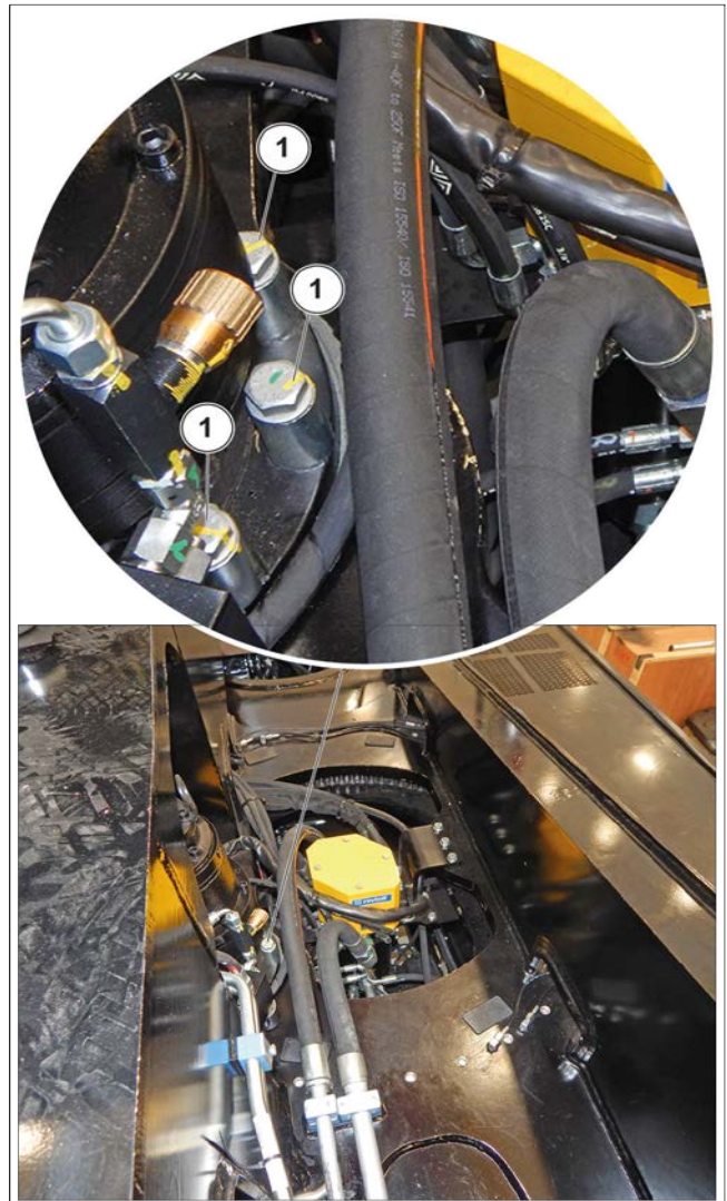
Figure 166: Rotation reducer fixing screw tightening check
