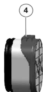
Figure 186: Dry air filter cartridge replacement 9643260EN-USMG(A/2021)
