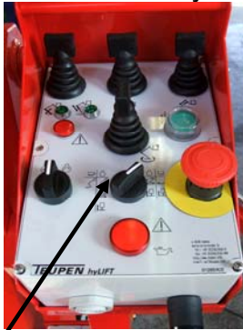
11. Selection switch: Position of stabilizing (quick moving)
